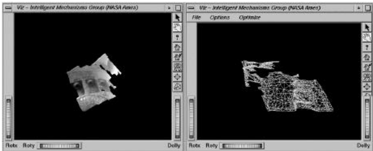
Figure 5.1 The Stereo Pipeline output from a single image pair taken using WAVE. Model on left is viewed with texture, the model on the right is the same model rotated 90 degrees and viewed as a wire frame.
